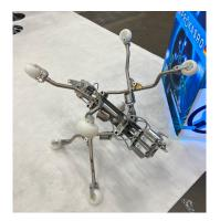
The KASRO UV Light Core DN 550-1200 employs electric motors to centralize within the sewer by adjusting expansion, monitored via a UV and heat-resistant pluggable camera in the core. Automatic shutdown prevents over-expansion at the preset diameter. Three cores can be connected for faster curing, and lamp performance can reach 12,000 W. For oval profiles like DN 500/DN 750, DN 600/DN 900, and DN 800/DN 1200, longer feet replace the two bottom feet, ensuring
